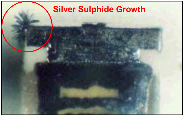
After sulphur testing (no KOA Resistor)
